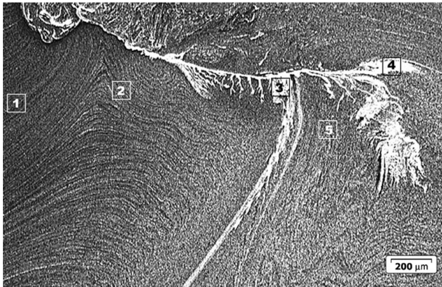
Figure 10 Light micrographs of transverse section (advancing side) through FSW produced in AA-8009 at a tool rotational speed of 1200 rpm and a traversing rate of 4.3 mm/s. DPH hardnesses associated with numbered locations are: #1—DPH 125; #2—DPH 131; #3—DPH 77; #4—DPH 54; #5—DPH 103; #6—DPH 105.
